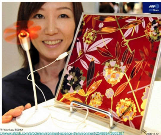
A dye-sensitized solar cell panel driving a fan from ambient light (courtesy Sony).
